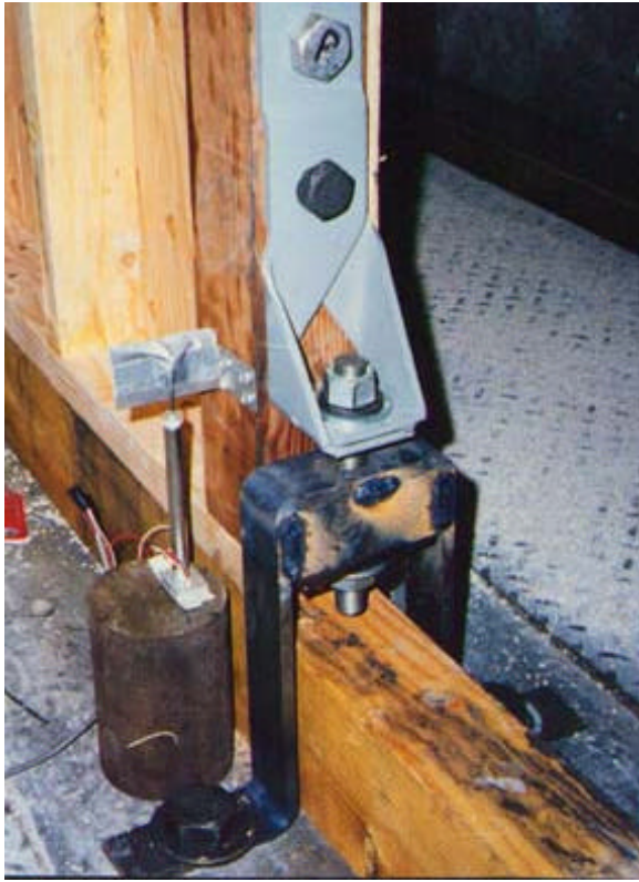
Figure 5, Hold down anchorage and Vertical deflectometer
