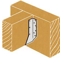
Projection seat for maximum bearing and section economy
